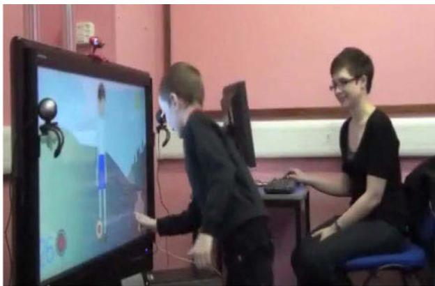
**Fig. 2** A child interacting with the ECHOES environment through touch. Three cameras are positioned on the sides and top of the screen, enabling real-time head position and eye gaze detection
